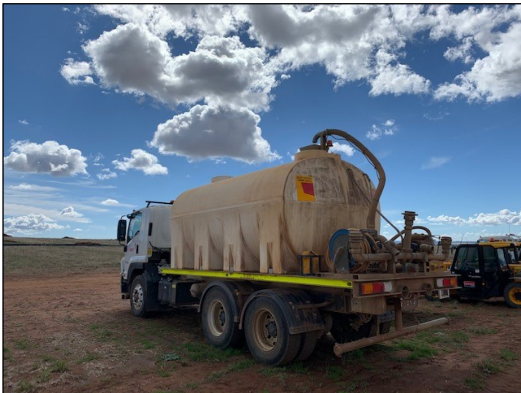
Plate 8: View of one (1) of five (5) site-based water carts used as part of the strategy to manage air quality during construction. No significant dust emissions were noted during site visit of 26/03/21.
